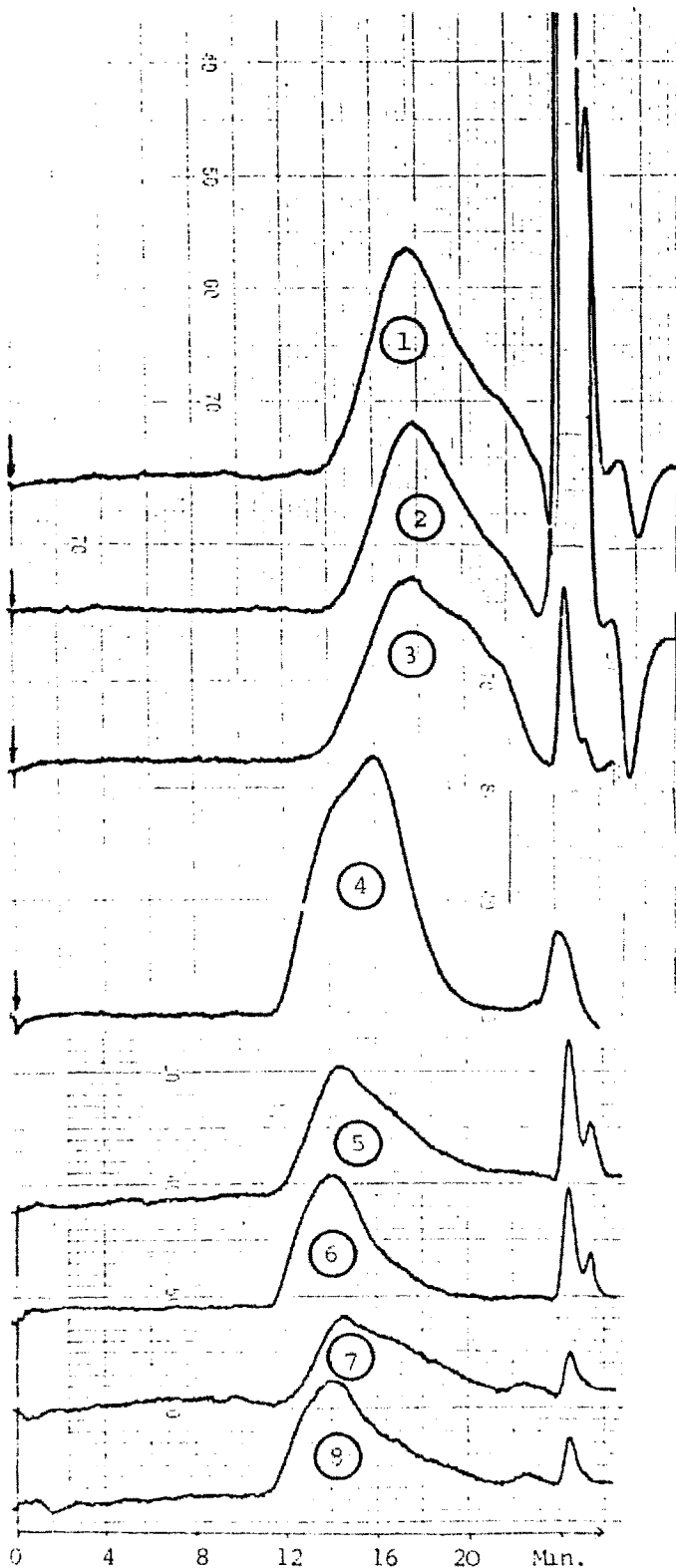
Fig. 2. Chromatograms of poly(methyl methacrylate) nanoparticles: \gamma -Ray initiated polymerization: (1) 100 mmol/l MMA a in phosphate-buffered saline, 4°C; (2) 100 mmol/l MMA a in water, 4°C; (3) 100 mmol/l MMA a in water, 4°C, freeze-dried. Commercial sample: (4) poly(methyl methacrylate) beads; diameter 10 \mu m. Chemically initiated polymerization: (5) 80 mmol/l MMA a in water, 3 mmol/l K 2 S 2 O 8 , 65°C; (6) 80 mmol/l MMA a in water, 0.3 mmol/l K 2 S 2 O 8 , 85°C; (7) 80 mmol/l MMA a in water, 3 mmol/l K 2 S 2 O 8 , 85°C. (8) 156 mmol/l MMA a in water, 3 mmol/l K 2 S 2 O 8 , 85°C.
